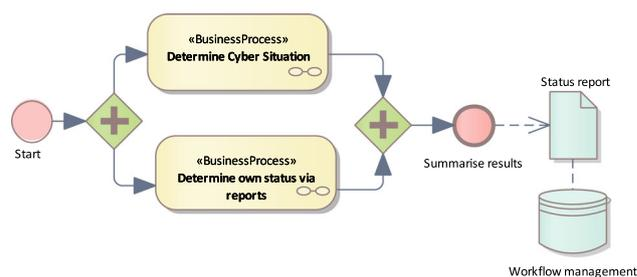
**Fig. 3** BPMN workflow: determine the overall security status (CCOP)
