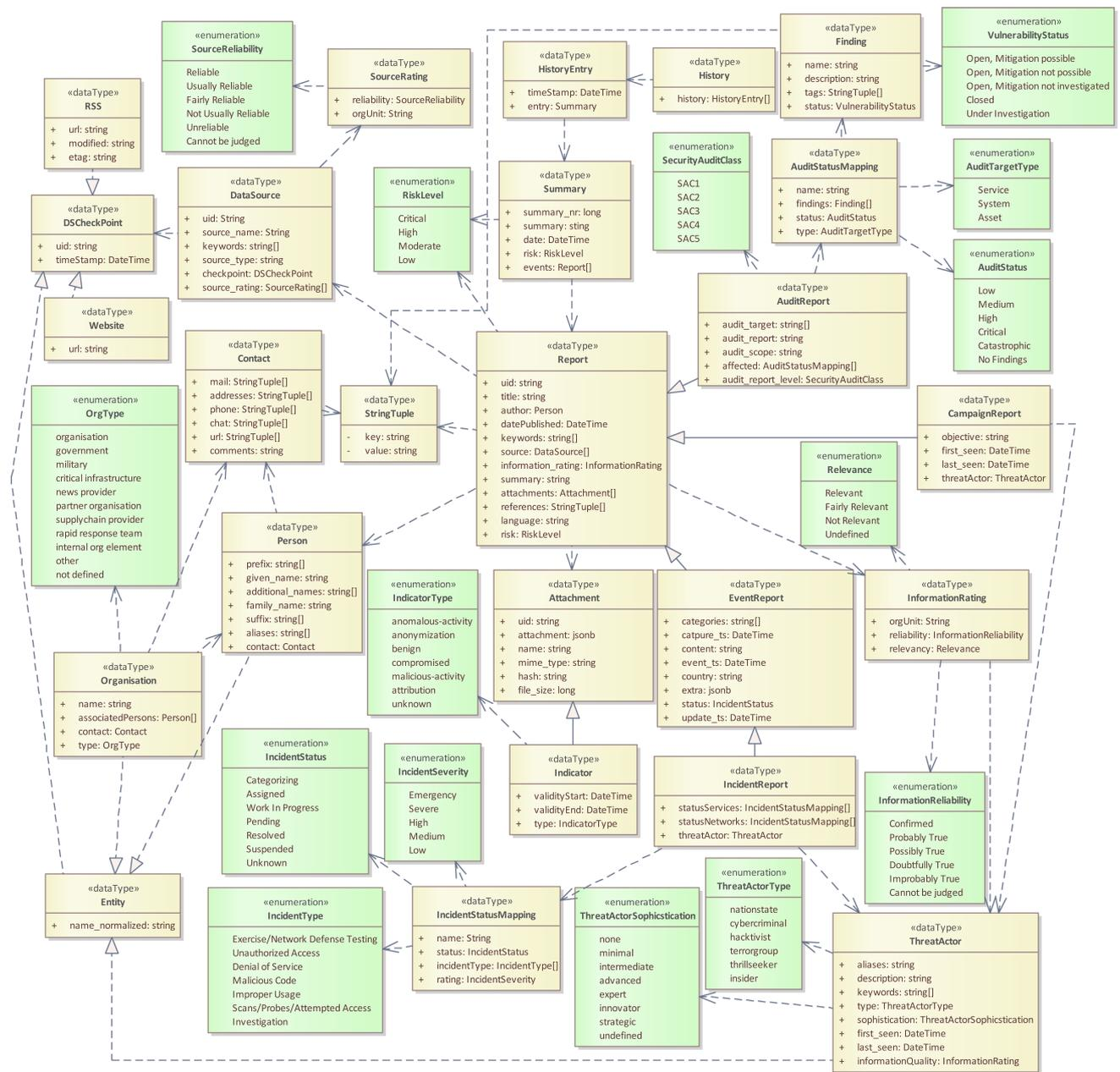
Fig. 2 Complete CCOP data model as UML class diagram
